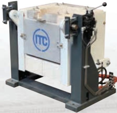
This induction melting furnace can melt 100lb./45kg to 1985lb./900kg of steel and 175lb./80kg to 2865lb./1300kg of brass. It has an extremely durable and high-quality construction with a cast and fired refractory top and bottom blocks. The induction coil is constructed from high-conductivity, heavy wall copper tubing. Power cables can be brought out by either side for better mobility. The floor mounted box furnace is installed onto stanchions.
