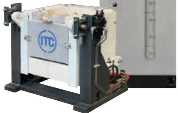
Equipped with one-man Nose Tilting furnaces, with a pneumatic assist for easy pouring, and a SmartPower™ system which allows the simultaneous melting of different metals. All while achieving zero down-time operation and reducing maintenance costs by utilizing the benefits of SmartPower™.
