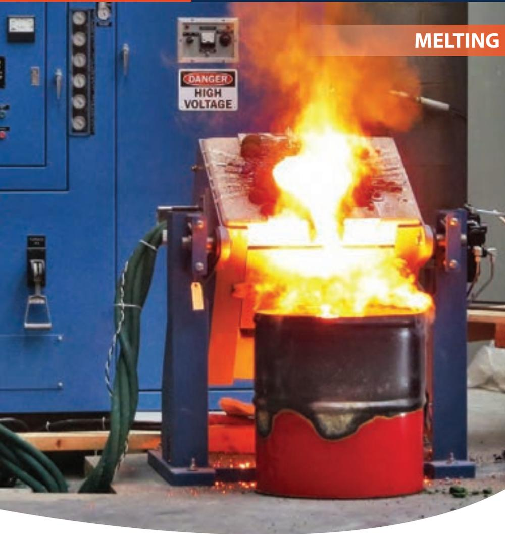
The melting furnace system is complete with power supply, hydraulically tilted furnace, removable steps and gates that open on either side of the platform for easy loading of pallets containing raw materials. This system can be easily designed to accommodate additional furnaces for alternate operation.
